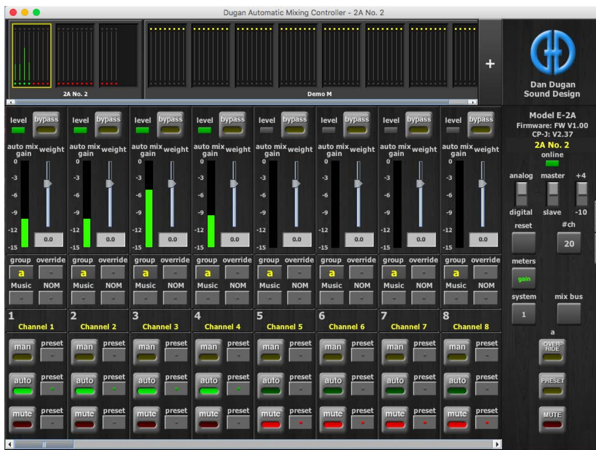
Figure 6-1 Dugan Control Panel
