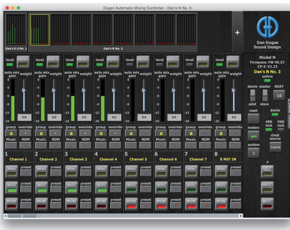
Figure 5-1 Dugan Control Panel
